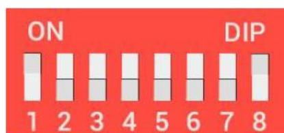
The CAN expansion module generally has an 8-code DIP switch used for communication configuration and resources mapping, dial ON to take effect, and the meaning of the DIP is as follows:
