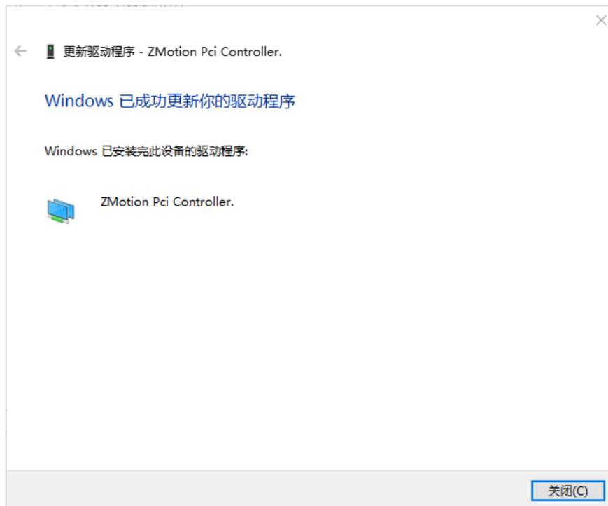
g. If there is "Zmotion Pci Controller" in the device manager, the installation is successful.
